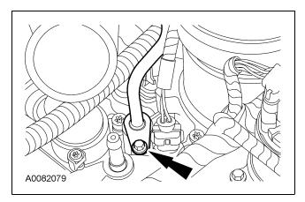
8. Remove the bolt and the wire retainer.
