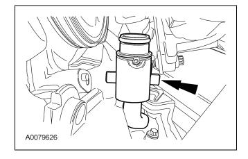
3. **NOTE:** Apply High Temperature Nickel Anti-Seize Lubricant to the bolt threads prior to installation.
