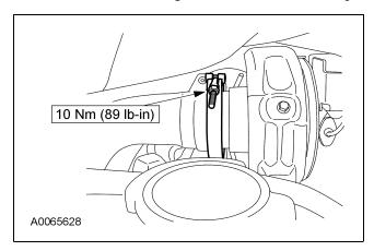
10. Position the wire retainer and install the bolt.
