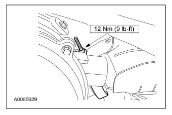
6. Position the clamp and tighten to specification.
