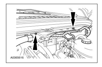
5. Disconnect the turbocharger variable vane hydraulic control valve electrical connector.
