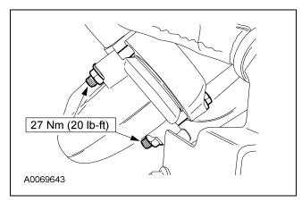
9. Install the turbocharger exhaust marmon clamp.
