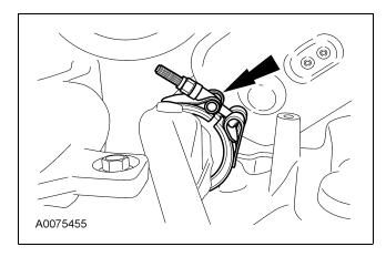
12. Loosen the LH exhaust inlet pipe-to-exhaust manifold nuts.
