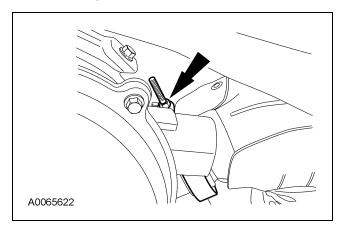
11. Loosen the exhaust inlet pipe-to-EGR cooler clamp.
