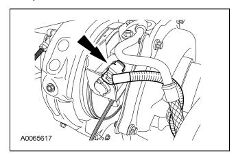
15. Position the wiring harness and connect the push pins.
