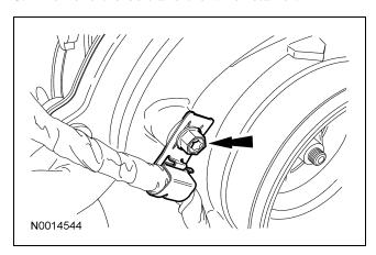
9. Remove the marmon clamp from the turbocharger outlet.
