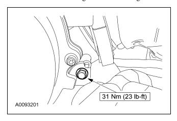
5. Install the turbocharger inlet marmon clamp.
