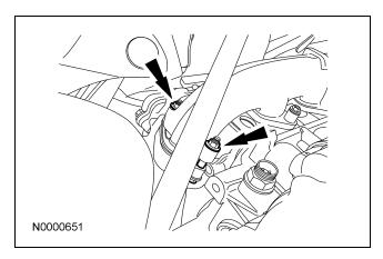
14. Remove the rear turbocharger mounting bolt.
