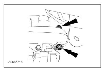
13. Loosen the RH exhaust inlet pipe-to-exhaust manfold nuts.
