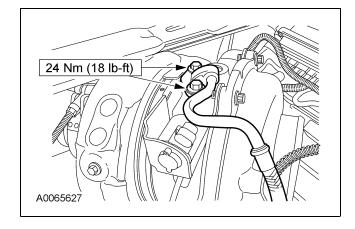
14. Connect the turbocharger variable vane hydraulic control valve electrical connector.
