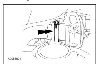
10. Remove the marmon clamp from the turbocharger inlet.
