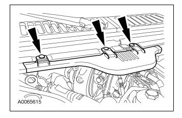
4. Disconnect the two wiring harness push pins and position aside.
