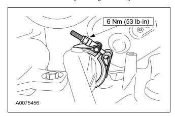
7. Make sure the exhaust inlet pipe is correctly aligned to the exhaust manifolds. Using hand tools, alternately tighten the nuts to draw the pipe to the exhaust manifold. There should be an equal gap spacing between the pipe flange and the exhaust manifold flange at the top and bottom bolts.
