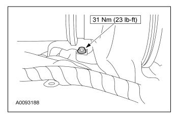
4. **NOTE:** Apply High Temperature Nickel Anti-Seize Lubricant to the bolt threads prior to installation.
