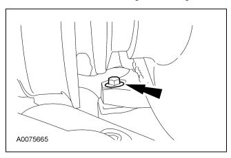
15. **NOTE:** Left side shown, right side similar. Remove the front mounting bolts.
